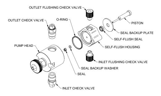
Figure 5-1. Stainless Steel Self-Flushing Pump Head Assembly
